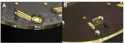
Centrifugal microfluidic devices also known as Lab-on-disc (LoD) platform, enables rapid assays in field forward settings. LoD platform requires simple equipment, such a rotating motor for sample preparation and actuation of fluidic within the disc via centrifugal forces. Moreover, this platform gives greater flexibility in embedding different sensors based on the chosen application.
